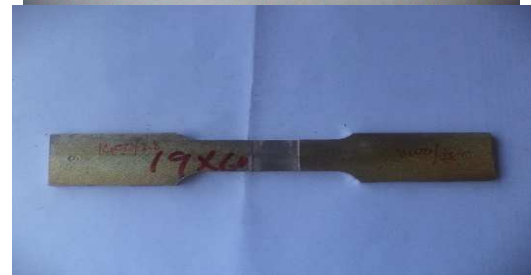
Fig 3: (a) Tensile specimen of FSW AZ31 at 1400rpm/26 mm/min. (b) at 1400rpm/28mm/min.
