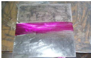
Fig.6. Die penetrant on with Copper Coated welded specimens
