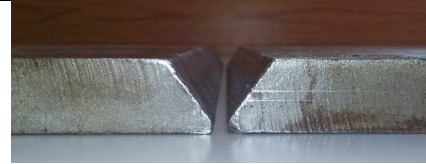
Fig. 2. Single V-notch Edge preparation carried out on 15CDV6 steel plates
