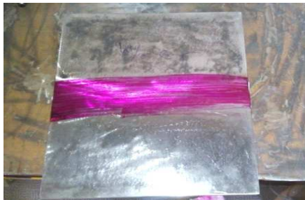
Fig.5. Die penetrant on without Copper Coated welded specimens
