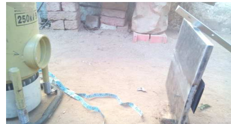
Fig. 7. Radiography Test On 15CDV6 welded specimen
