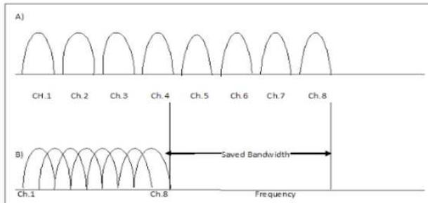
Figure 2.4: (A) and (B) conventional FDM and OFDM.
