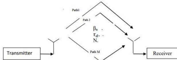
Figure 3.1: Multipath fading channel.
