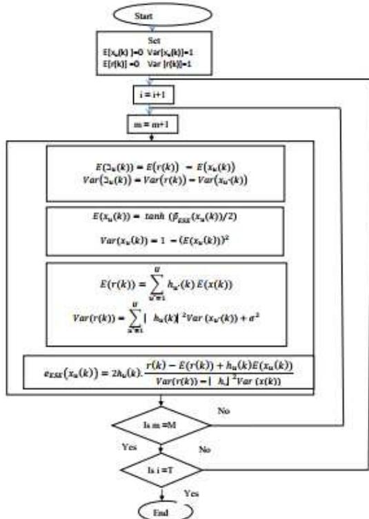
Figure 2.10: Chip-by-chip detection flow chart for IDMA system
