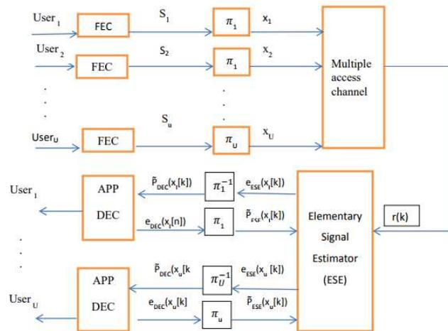
Figure 2.9: IDMA transmitter and receiver structure.
