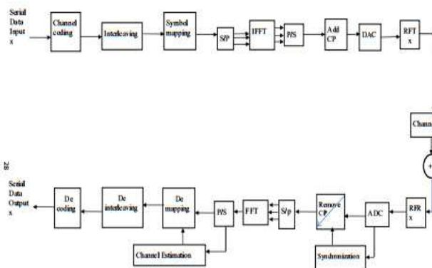
Figure 2.6: Block diagram of a baseband OFDM transceiver
