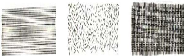
Fig.2. Continuous, chopped and woven fibrous composite materials
