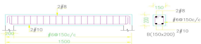
Figure 1: Reinforcement details of the beam
