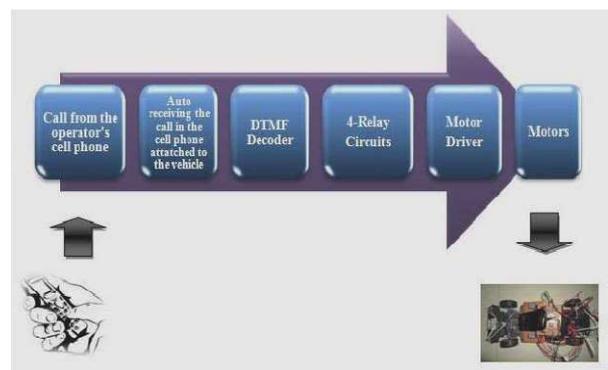
Figure.1. Block diagram of GSM network controlled vehicle.
