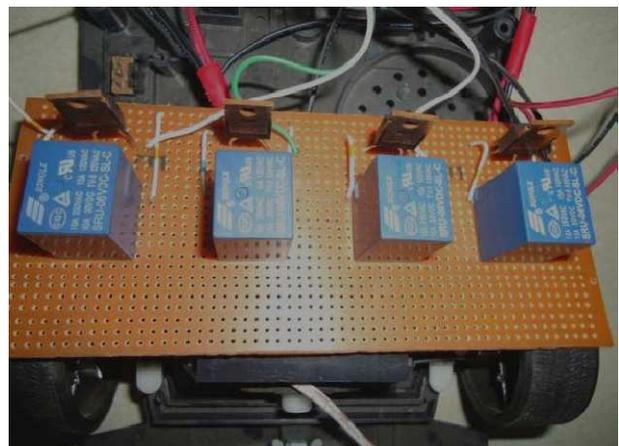
Figure.4. Relays implemented on vero board
