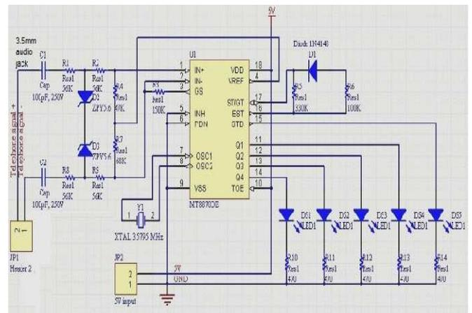
Figure.3. Connection diagram of DTMF circuit
