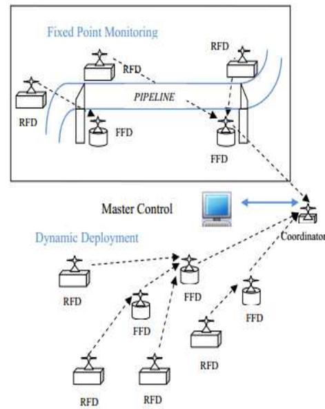
FIG: represent the sensor node structure consists of two sections - dynamic deployment and fixed point monitoring.
