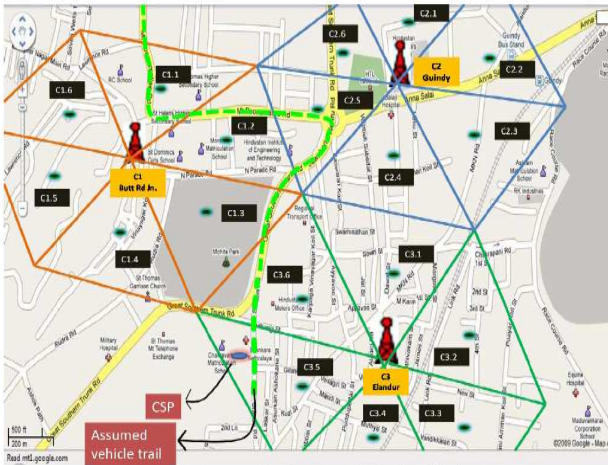
Fig. 7. Actual GSM tower position and zone tags marked on the road map of the region.
