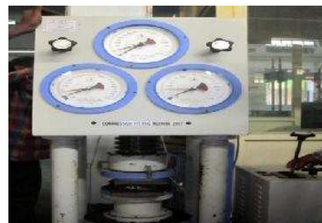
Figure 3 Compression Tests of Metallurgical Dust Briquettes
